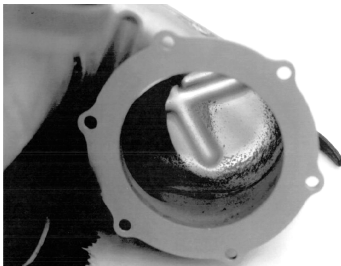
Figure 1.—Cabin air return duct in Apollo 11 command module after return to Earth.
