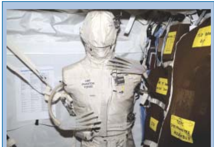
The Phantom Torso, seen in the Destiny laboratory on the International Space Station. The torso is designed to measure radiation dose throughout the human body. It was delivered to ISS by the STS-100 crew in April 2001. (NASA photo ISS002-E-5952.)
